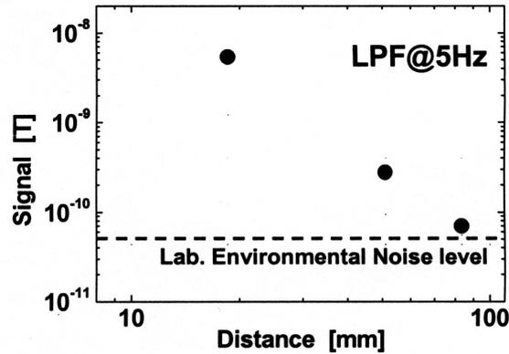
FIG. 9: Magnetic signal vs. distance. The signal intensity is inversely proportional to the cubic of distance.
