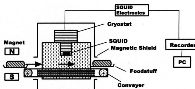
FIG. 1: Block diagram of food contamination detection system. It consists of a permanent magnet, a conveyer, a magnetically shielded box and SQUIDs.
