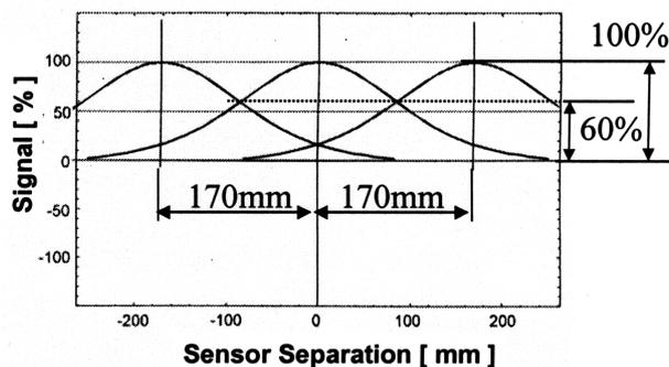
FIG. 3: Distribution of SQUID sensitivity. Sensitivity more than 60% of maximum value can be obtained in any place on the conveyer with 500 mm width if three SQUIDS are employed.
