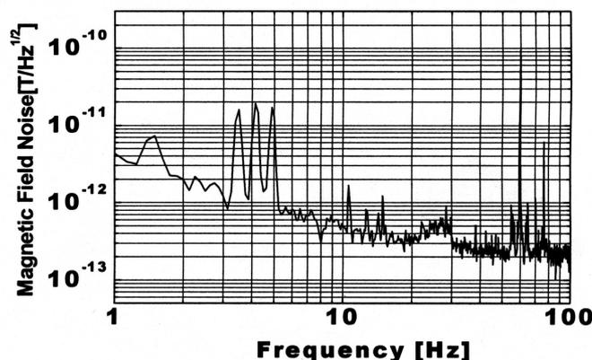
FIG. 5: Noise spectra of the system. Several peaks around 3 to 5 Hz are due to the environmental noise at the laboratory. The peak at 60 Hz is from the appliance frequency. The noise at 10 Hz is 300–400 fT/Hz<sup>1/2</sup>.
