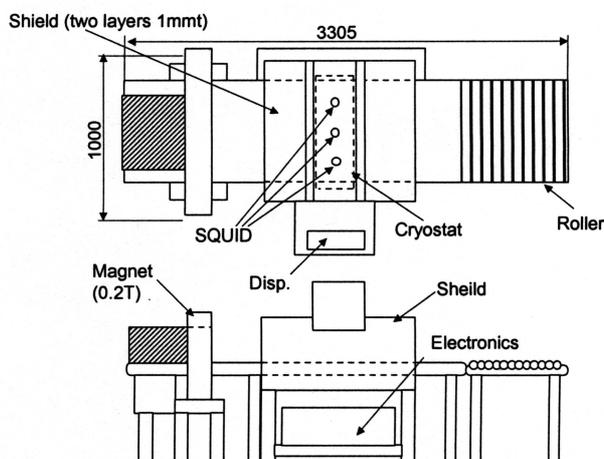
FIG. 4: Design drawing of the large system for meat block. The size is 3305L×1290W×1610H.
