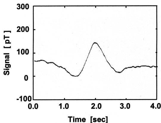
FIG. 6: Time trace of the detected signal. A cut stainless steel syringe needle with dimension of  $0.9 \times 2$  mm was measured. The distance between the test piece and the SQUID sensor was set at 200 mm.
